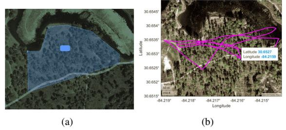
Fig. 5. Deploying an UAS in a prescribed burn to collect environment data. (a) The prescribed burn area (highlighted with the blue color). (b) The flight trajectory of the UAS, where the UAS is controlled by the human operator. The labeled position in the diagram is the start position.
