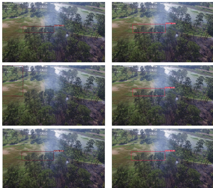
Figure 8. The figures on the left are the YOLOv7 bounding box detection on Frames 756, 757, and 758. The figures on the right are the Algorithm 1 bounding box prediction on Frames 756, 757, and 758.
